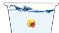
IP67: Submersion to one meter for 30 minutes.
